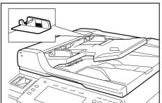
Ensure that loaded originals do not exceed the level indicator. If exceeded, originals may jam (see the figure).
